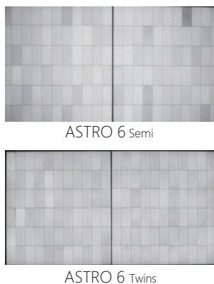
Elimination of ASTRO 6 cracks in mechanical load test
