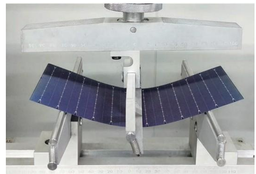
Three-point bending test of cell
